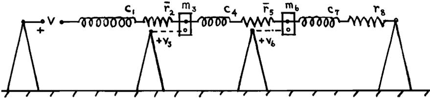
FIG. 10. Mechanical system.
